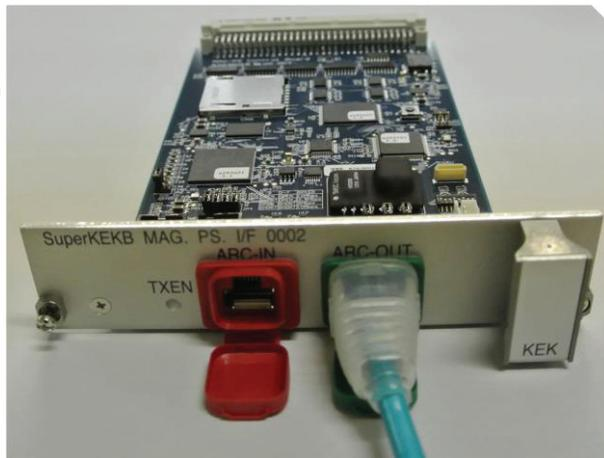
Figure 5: Prototype of the new PSICM.
