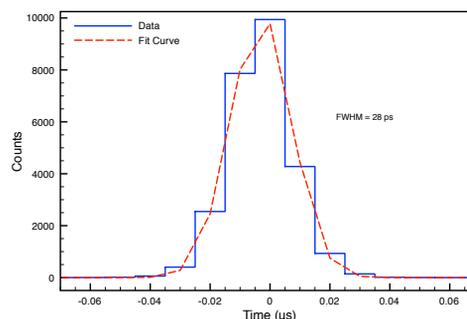
Figure 3: Time dispersion obtained using a pulse generator sending the same pulse on 2 different digitiser channel.
