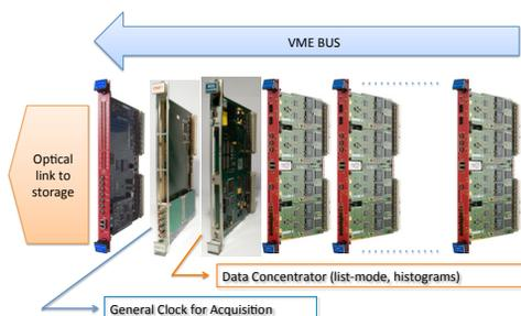
Figure 2: Layout of the digital acquisition chain.
