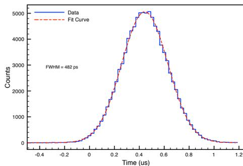
Figure 4: Time dispersion obtained with two LaBr<sub>3</sub>(Ce) detectors placed in front of a <sup>22</sup>Na source.
