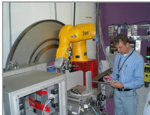
Figure 1: Shows the sample table (center, low), the detector assembly (left), the robot arm (center, yellow), the neutron beam orifice (right, back) and user (Jim).
