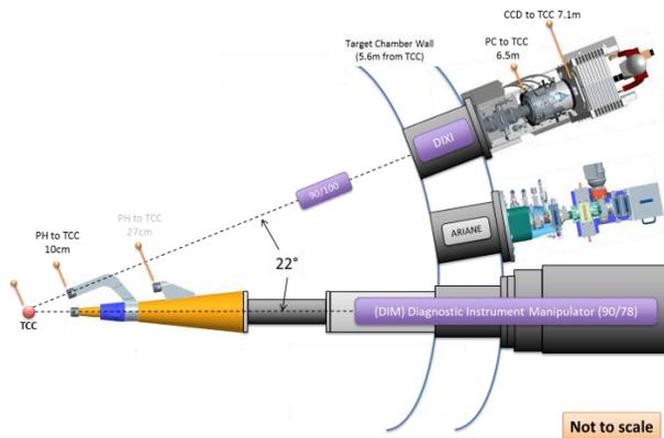
Figure 2: System layout of DIXI Diagnostic in NIF.
