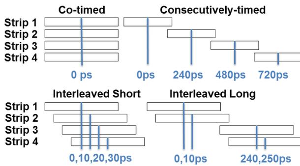
Figure 5: Proposed DIXI timing setups for NIF.
