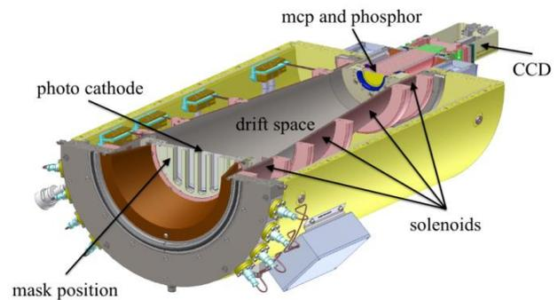
Figure 4: Cutaway detail of DIXI instrument.
