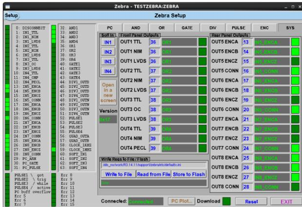
Figure 5: EDM screen showing wiring of output signals.
