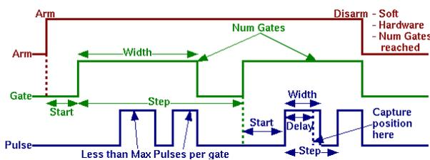
Figure 2: Arm, Gate and Pulse signals of ZEBRA position capture block.
