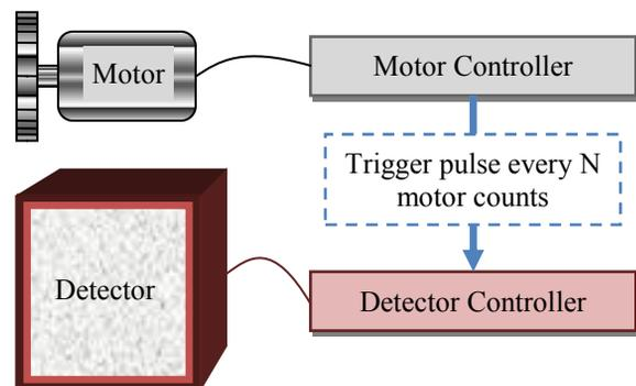
Figure 1: Sample experimental setup.
