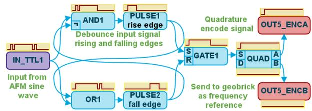
Figure 6: Diagram of chopper logic block connections.
