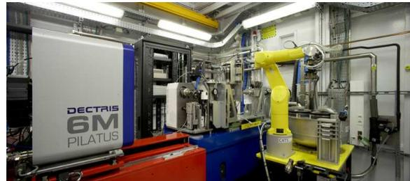
Figure 1: XALOC end station, main components (left to right): detector (on red table), goniometer and beam conditioning elements (on blue table), and automatic sample changer (yellow).
