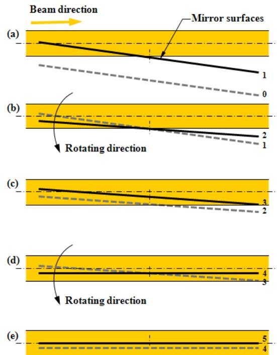
Figure 2: Process of achieving the half-cut state of a mirror.
