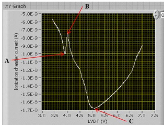
Figure 4: Variations in the IC outputs with respect to the pitch angles of the VFM.
