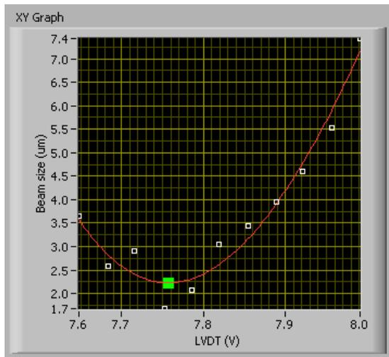
Figure 3: Graph of the beam sizes measured at equally partitioned positions within the interval containing the pitch angle corresponding to the minimum beam size.
