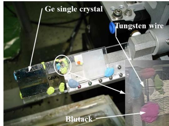
Figure 1: The sample holder and a close-up view of the tungsten wires.
