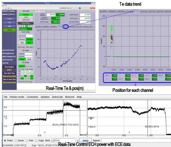
Figure 4: OPI panels to operate DAQ system and display electron temperature data in run-time, result of ECH power control on real-time with ECE.
