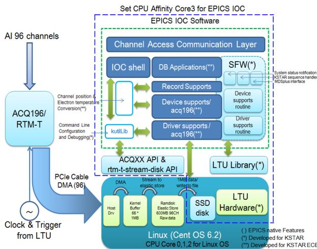
Figure 2: Function blocks for ECE IOC.
