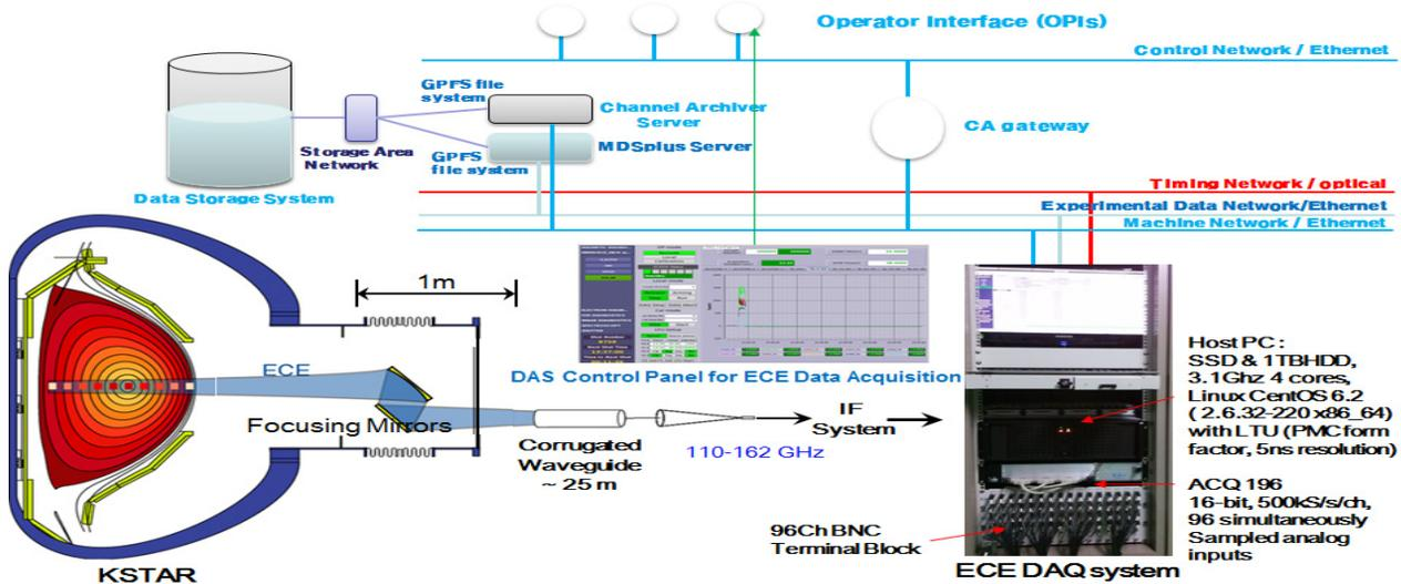
Figure 1: Network connections to the infrastructure of the KSTAR control system and Configuration of ECE DAQ System.
