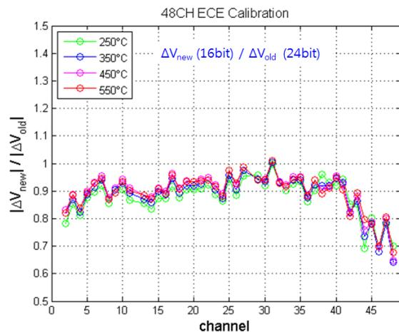
Figure 3: Comparison of calibration factor between new and old DAQ.
