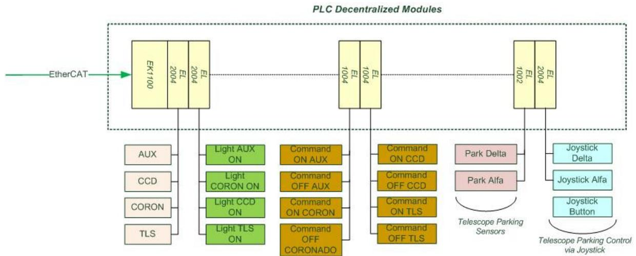
Figure 4: Functions controlled by the PLC modules in the telescope room.
