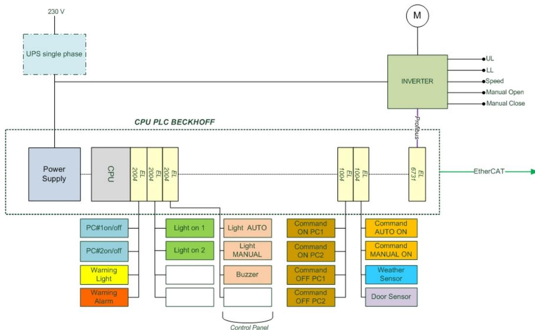
Figure 3: Functions controlled by the PLC modules in the control room.
