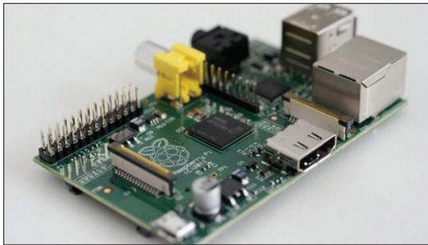
Figure 3: Raspberry Pi computer board (model B, rev. 2).
