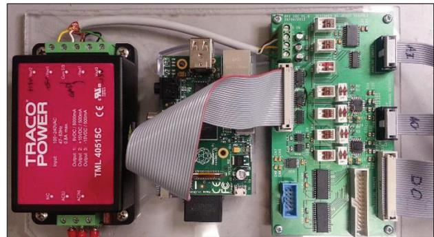
Figure 8: EPICS IOC for the control of the focalization system.
