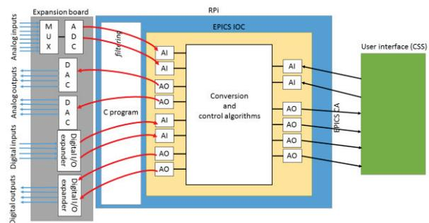
Figure 4: Interface between the EPICS IOC records and the expansion board using a C program.
