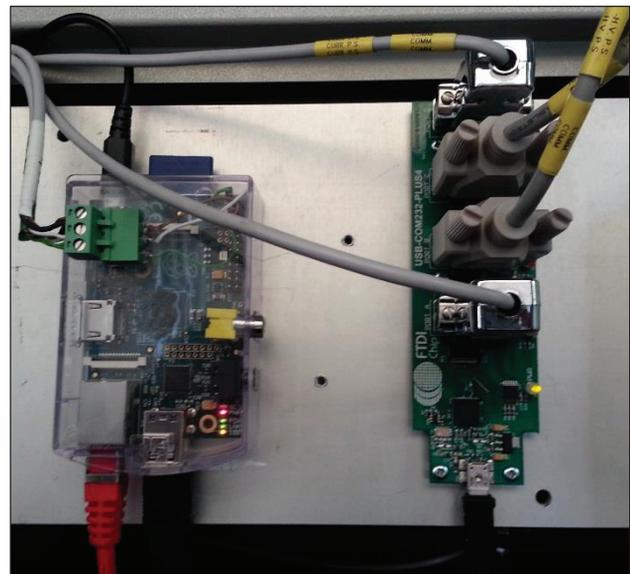
Figure 7: EPICS IOC for the control of the mass separator.
