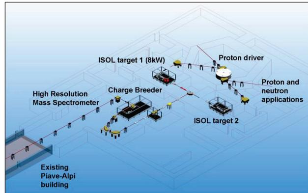
Figure 1: The SPES facility layout.
