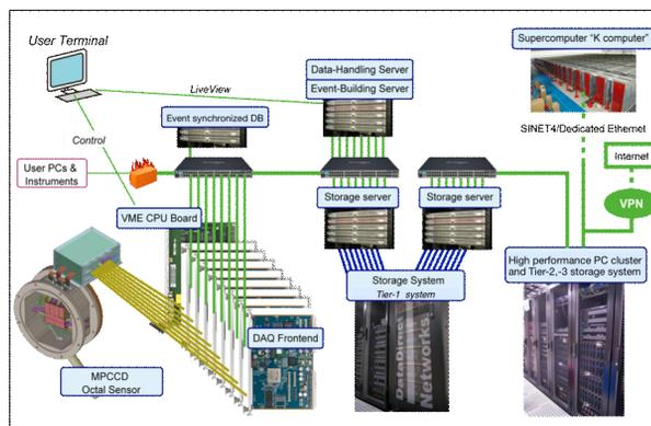
Figure 1: Overview of the DAQ system. The current DAQ system supports up to 10 multi-port charge-coupled device sensors.
