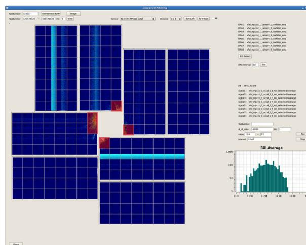
Figure 4: GUI image of the low-level filtering system. The region to the left shows MPCCD image data. A histogram of the ROI average photon number is shown in the lower right.
