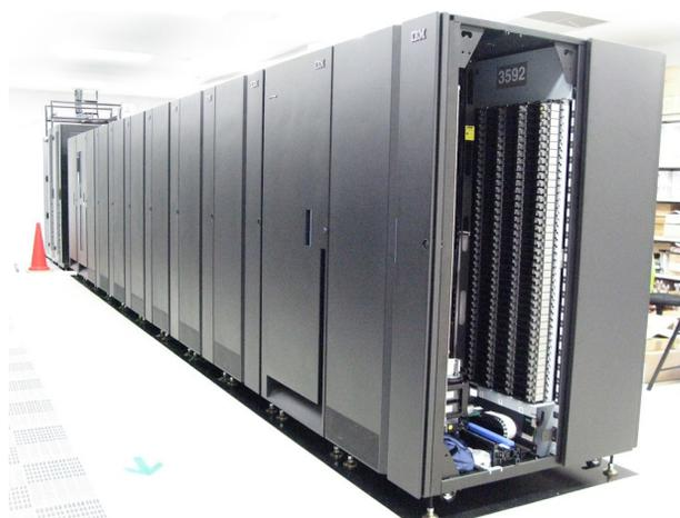
Figure 3: Long-term storage system installed in the SACLA computer room consisting of a 1 PB disk array and 6 PB tape library.
