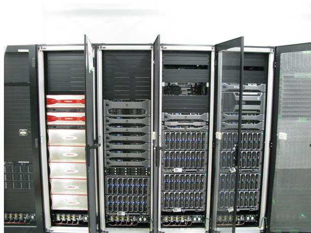
Figure 2: High-performance computing system installed in the SACLA computer room. The HPC system consists of an 80-node cluster system and a single-node SMP system.
