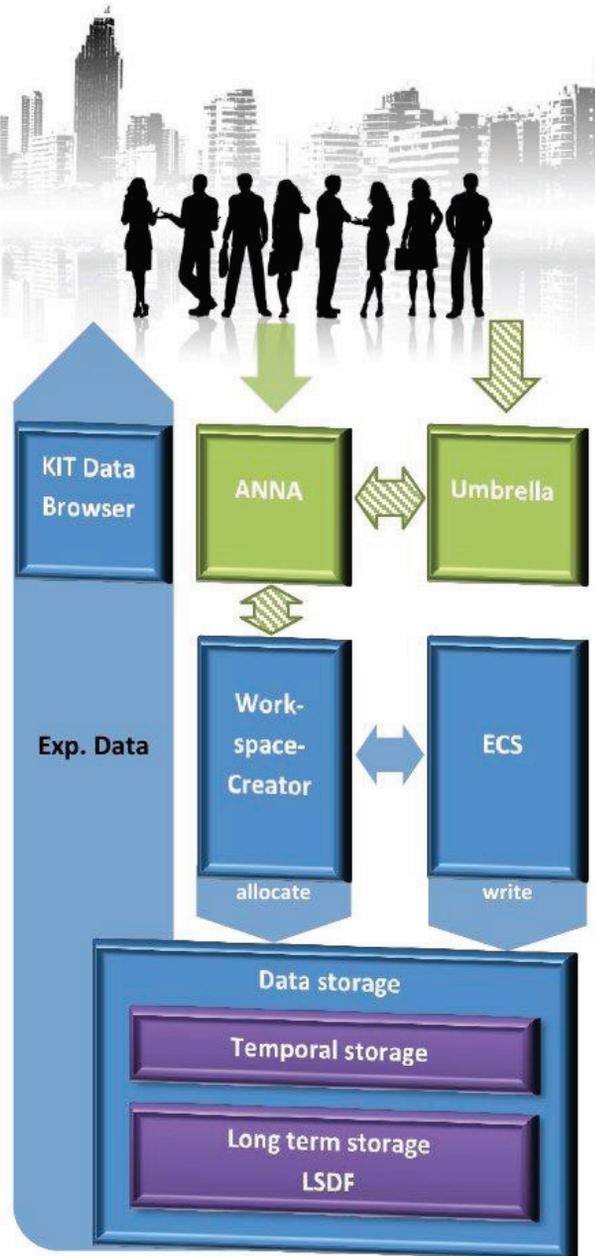
Figure 4: Schematic concept of the dataflow between the different parts of the Tango based control system (the dashed parts are in development).
