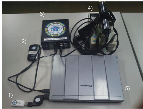
Figure 2: The in-vehicle part is compactly composed of mostly commercial components. 1) GPS unit, 2) 3G mobile wi-fi router, 3) MAKUNOUCHI, 4) NaI survey meter, 5) PC.
