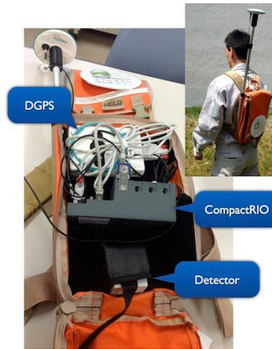
Figure 11: KURAMA-II for the measurement on foot. In this case, a differential GPS (DGPS) unit is used to achieve high accuracy (around 1 m) of positioning sufficient for walking survey.
