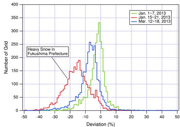
Figure 8: The deviation of air dose rate from the reference period (from Dec. 20 to 31, 2012) in Fukushima monitored by KURAMA-II on city buses. Heavy snow greatly reduced the air dose rate by shielding the radiation.
