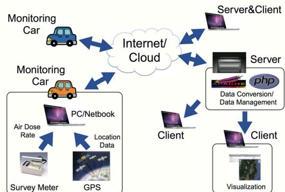
Figure 1: KURAMA system. Monitoring cars and servers are connected over the Internet by cloud technology.
