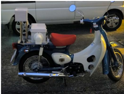
Figure 10: KURAMA-II on a motorcycle. A CsI detector and other components are separately placed in polycarbonate boxes. The height of the detector is adjusted to 1 m above the ground, to meet the standard for the air dose measurement in this accident.
