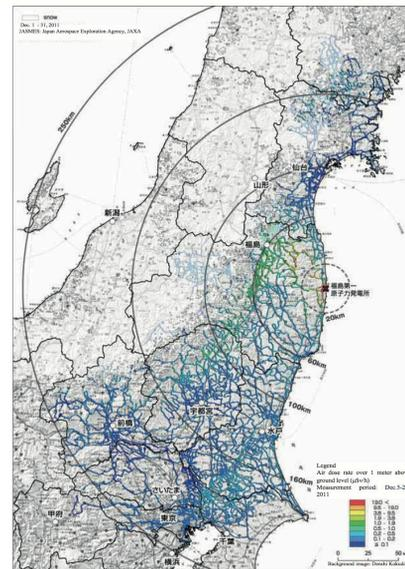
Figure 4: The air dose rate mapped by KURAMA in Dec. 2011 [4]. MEXT performed the first and second carborne surveys of the East-Japan by KURAMA in June and December 2011, respectively.
