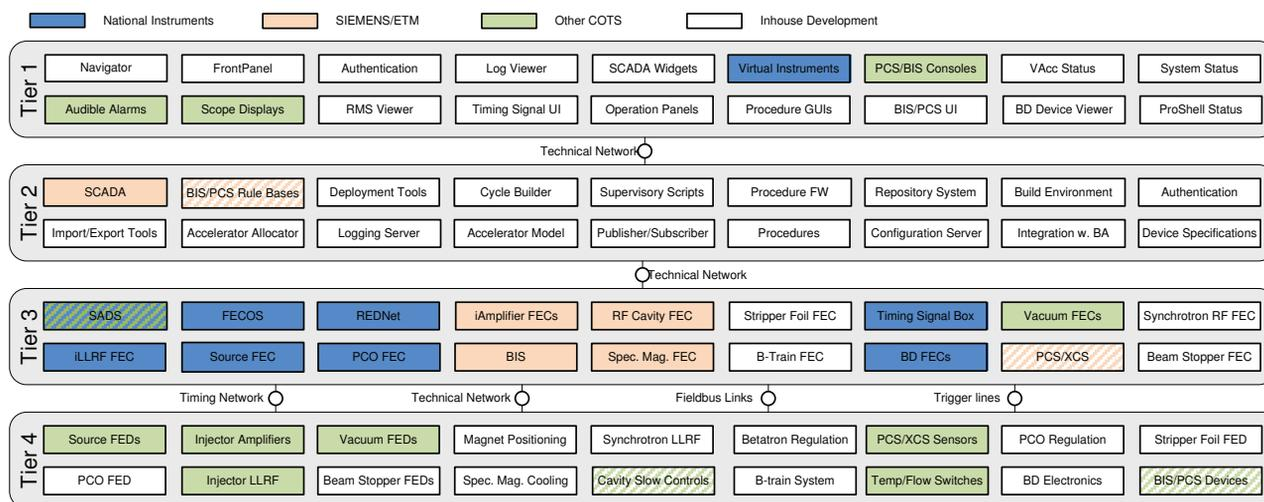
Figure 3: Accelerator control system components at four individual tiers.
