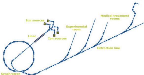
Figure 1: Layout of the MedAustron accelerator.
