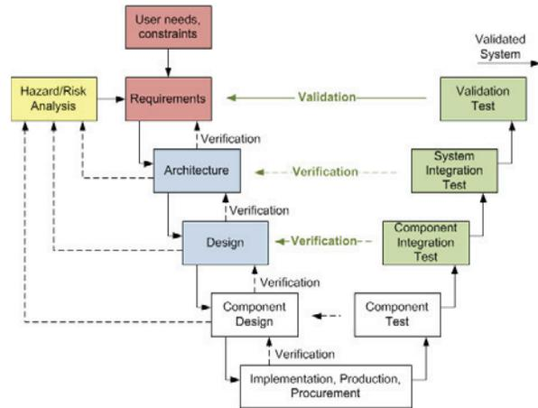
Figure 2: V-model applied for systems engineering process as taken from EN 61508 and EN 62304.
