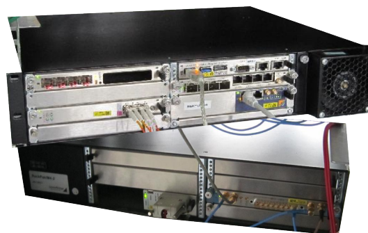
Figure 2: XFEL GUN mTCA.4 LLRF system in 2U crate.
