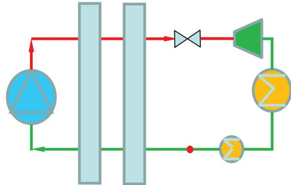
Figure 1: Diagram of a large scale helium refrigerator.
