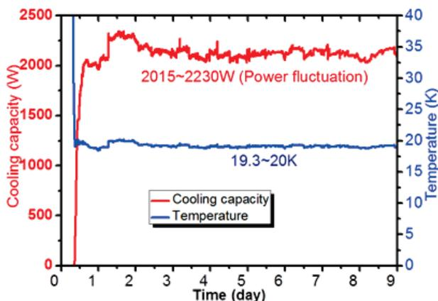
Figure 5: Long period temperature stability of operation situation for the large scale helium refrigerator.
