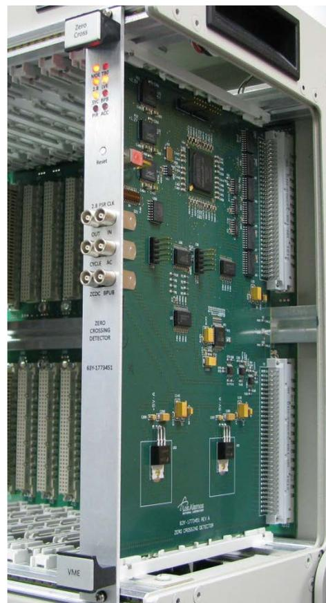
Figure 2: The LANSCE timing reference generator.
