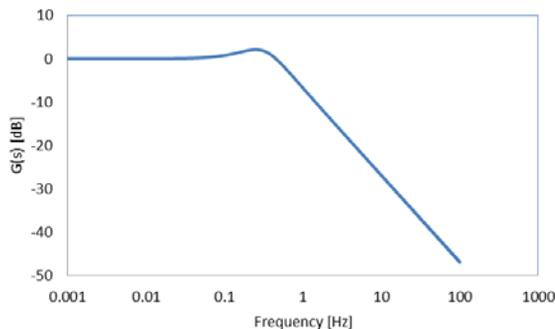
Figure 4: Transfer function for this PLL.
