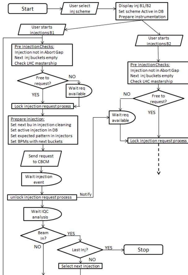
Figure 2: Simplified flow chart of the injection process.
