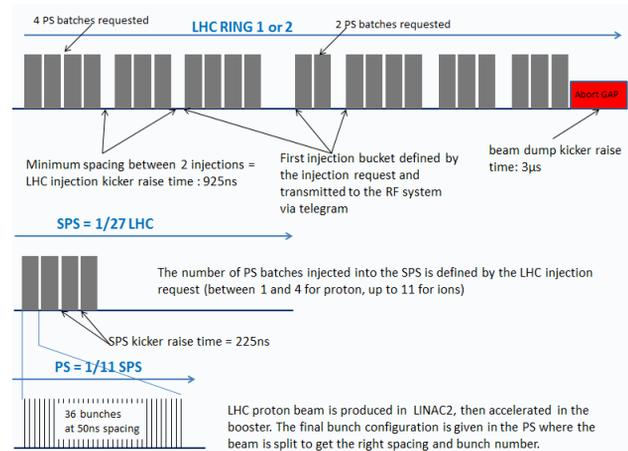
Figure 1: LHC injection scheme.
