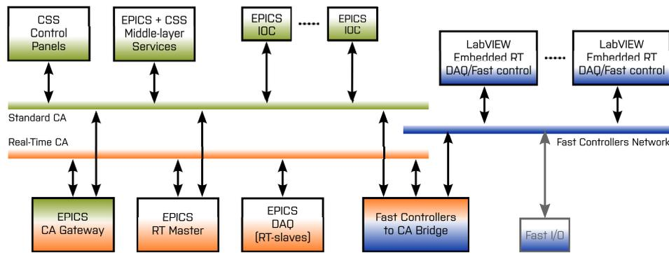
Figure 1: Proposed control system SW architecture including EPICS and LabVIEW controllers.
