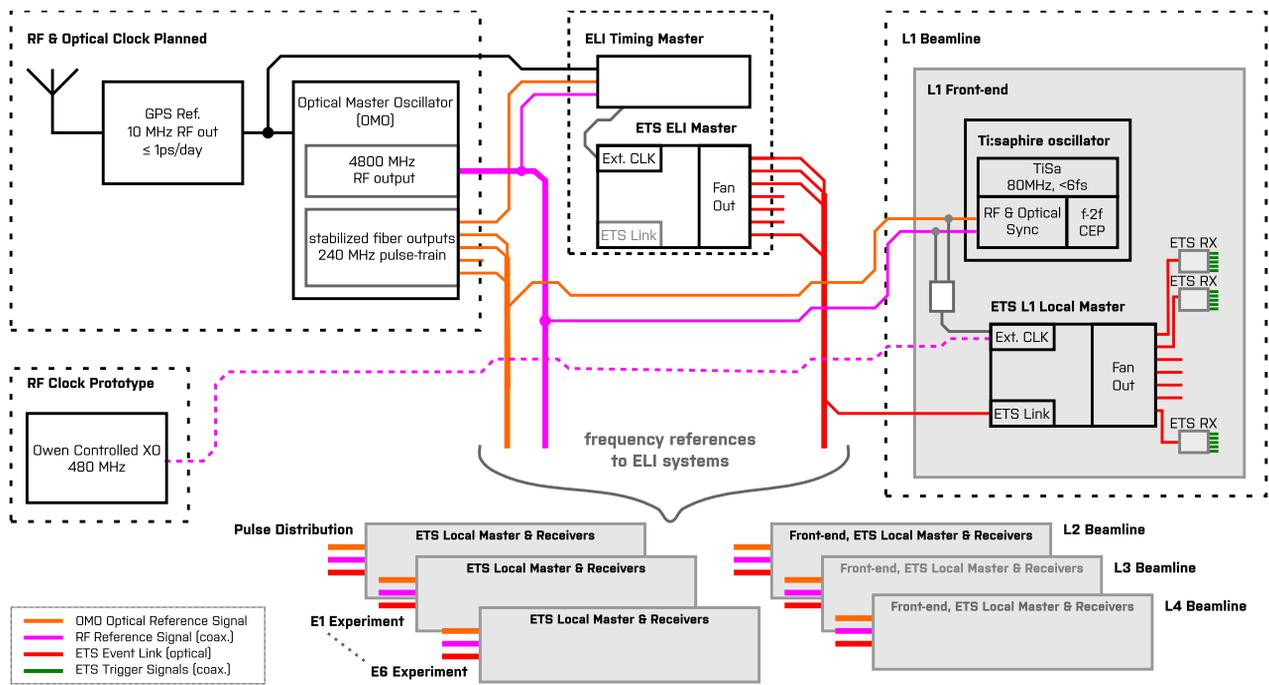
Figure 2: Timing and frequency synchronization scheme.
