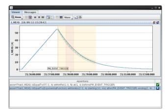
Figure 1: The display of an analysis result consists of a list of assertion lines, and a chart showing the detail of the selected line. The graph highlights the area covered by the assertion in orange and the failing part in red.
