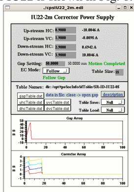
Figure 6: Local compensation prototype for IU22.
