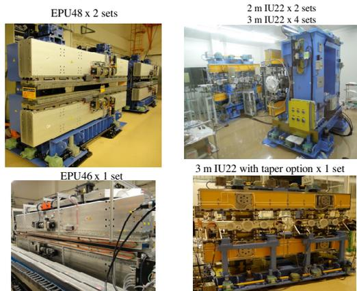
Figure 1: Insertion devices of TPS in the phase-I.
