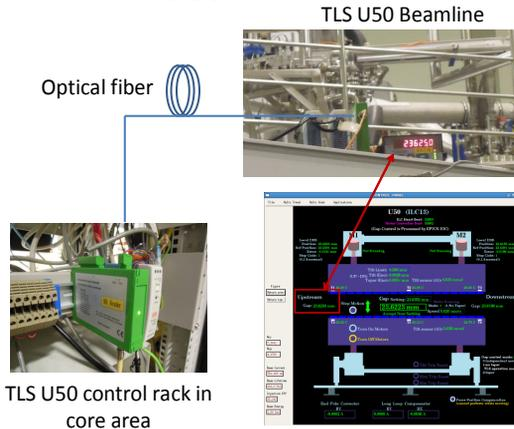
Figure 11: Gap value of U50 for on-the-fly experiments via directly send SSI encoder hardware signals through fibre link in TLS.
