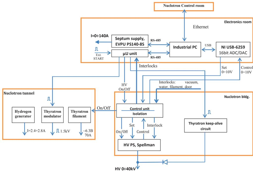
Figure 2: Nuclotron injection control system structure.
