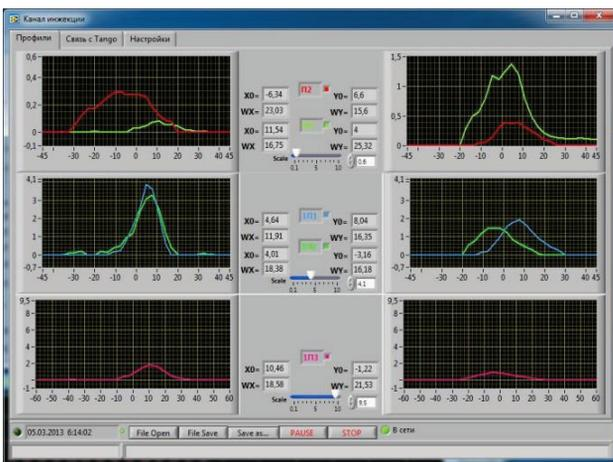
Figure 5: Transversal beam profiles in the transfer line.
