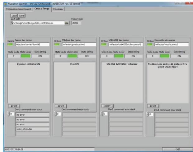
Figure 4: Injection control client application.
