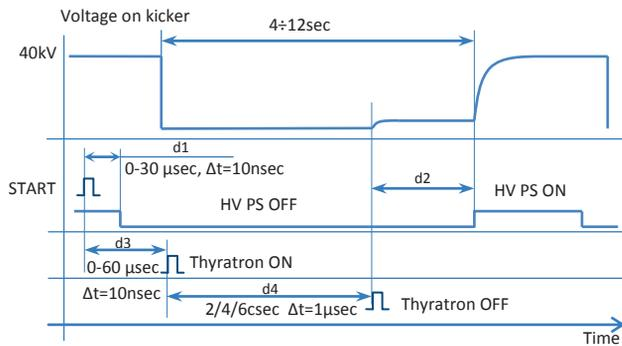
Figure 3: Electrostatic kicker supply time diagram.
