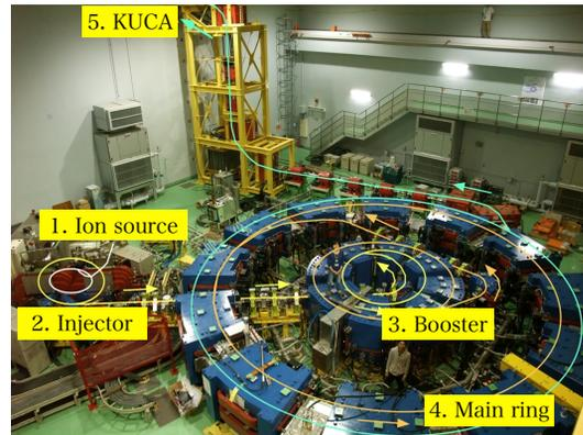
Figure 1: The initial FFAG accelerator complex in KURRI.
