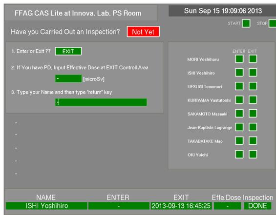
Figure 7: Access control for the radiation controlled area.
