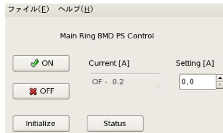
Figure 4: Operator Interface developed with GTK for the MR defocusing magnet control.
