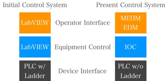
Figure 5: Comparison of standard design between initial control system and present one
