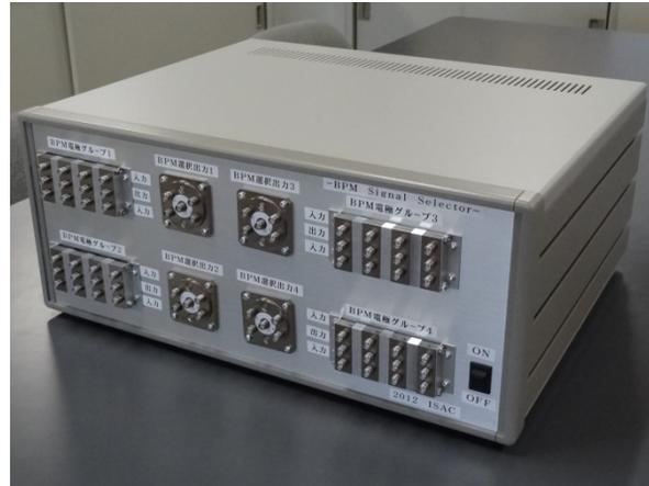
Figure 1: Signal switching box (front view).
