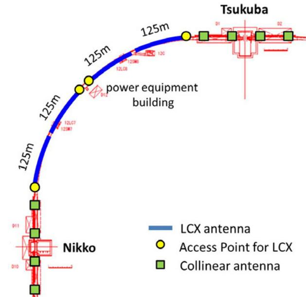
Figure 6: Layout of the wireless LAN components in the SuperKEKB tunnel. Blue lines, yellow circles, green squares indicate the LCX antennas, access points for LCX, and collinear antennas, respectively. The figure is for the 1/4 of the SuperKEKB main ring.
