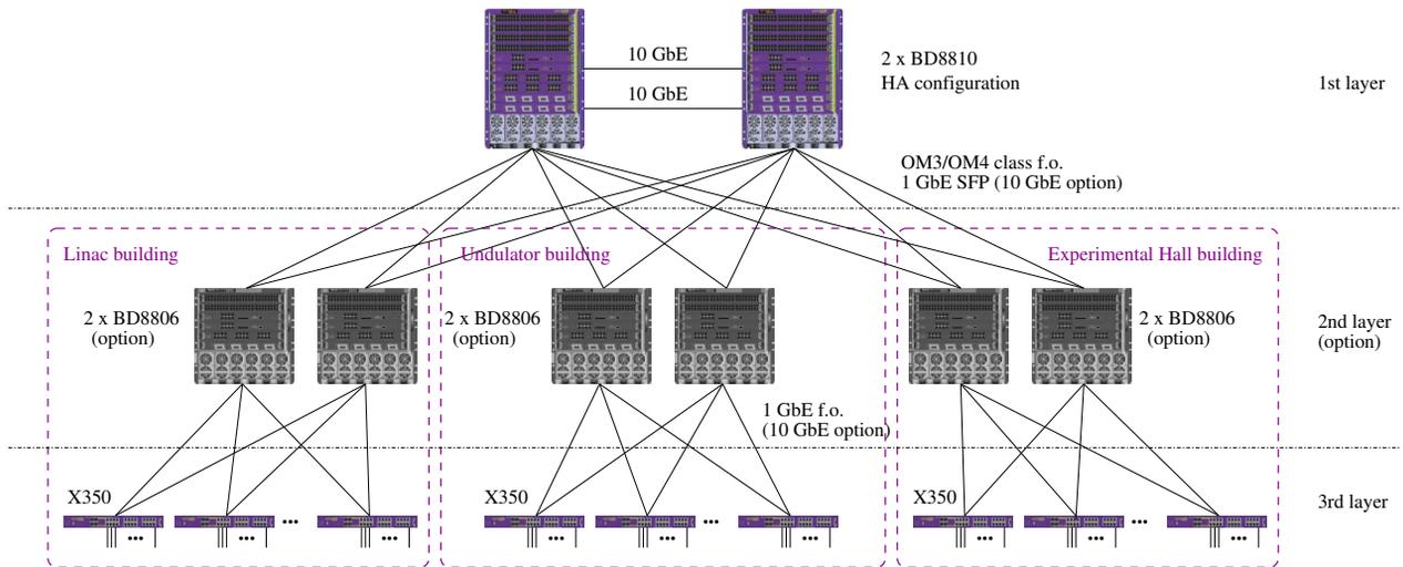
Figure 1: Controls network layout. Local network segments not shown.
