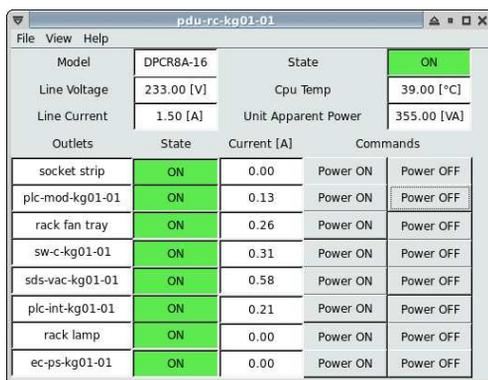
Figure 3: PDU graphical user interface.
