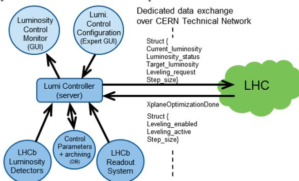
Figure 1: Block diagram of the LHCb luminosity control.
