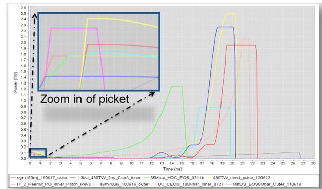
Figure 2: Example of pulse shapes for different experiments. Both small features (picket) and larger scale features must be accurately shaped.
