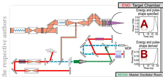
Figure 1: A sample beam line layout with Master Oscillator Room (MOR) at the beginning (B) and Target Chamber at the end (A).
