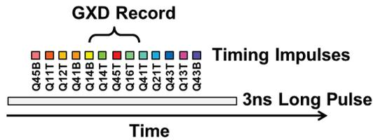
Figure 4: Beam timing for cross-timing shot with pointing as shown in Figure 3. The GXD trigger is set to image signals from the quads indicated by the braces.
