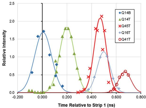
Figure 6: Intensity histories for the x-ray spots indicated in Figure 5. Signal levels from the individual images are plotted as points, and Gaussian fit profiles are indicated with solid lines.
