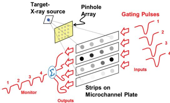
Figure 1: Gated X-ray Detector principle of operation. See text for details.
