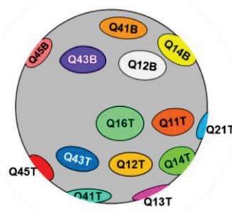
Figure 3: Typical beam pointing for cross-timing shot as viewed from the equator of the target chamber at 78° azimuth. All 4 beams in each quad are pointed to the same spot.
