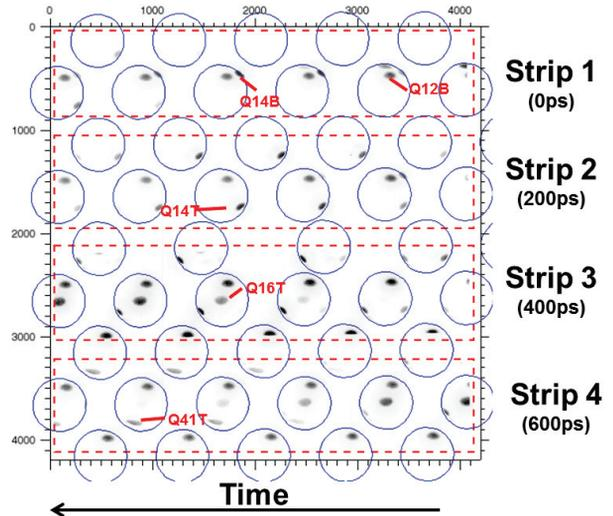
Figure 5: GXD image from timing shot N130117. Strip boundaries are indicated by red dashed lines, and the gate travel is from right to left. The strips were delayed in 200ps intervals as indicated. The outline of the spherical target within each pinhole image is indicated in blue.
