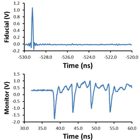
Figure 2: A two-channel digitizer record showing the fiducial reference pulse (top) and the GXD monitor signal (bottom). The negative pulses correspond to the time-multiplexed gate pulses that propagated through strips 1 through 4, respectively.
