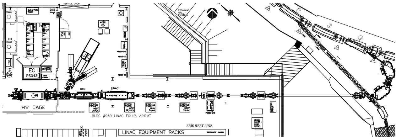
Figure 5: Layout of EBIS, from ion sources (the planned Laser Ion source is shown between the two ion sources) to booster injection.
