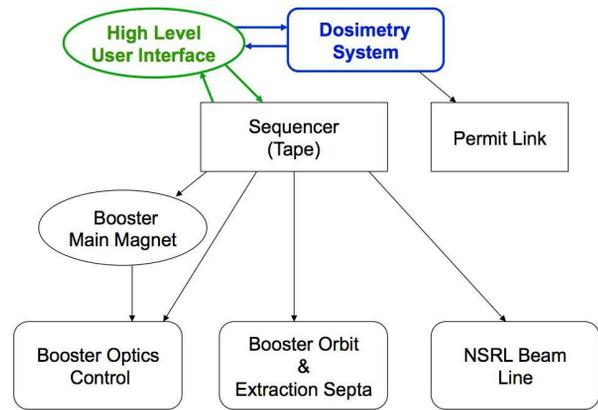
Figure 2: Block diagram of the controls for the SPE simulator. A sequence is defined for a set of requested beam energies. The dosimetry system, a part of the NSRL target monitoring systems, signals when the desired exposure has been achieved for a given energy and a new energy is selected in the sequence. Note, the lines between the Dosimetry system and the high level interface are not implemented for the SPE simulator, but will be for the GCR simulator.
