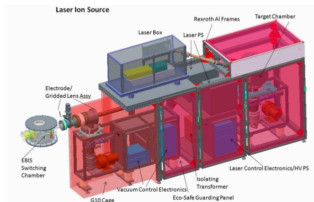
Figure 4: Layout of the Laser Ion Source. The laser, sitting above the beamline in the diagram, sends a laser pulse down into a chamber with a target holder that contains many different solid targets.
