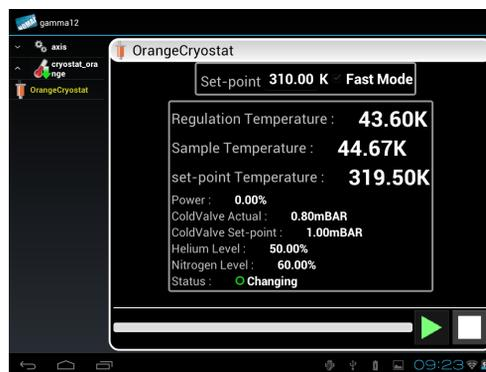
Figure 5: Example of the Orange Cryostat control screen.
