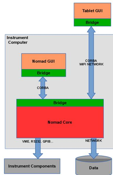
Figure 1: Layout of the various NOMAD components.
