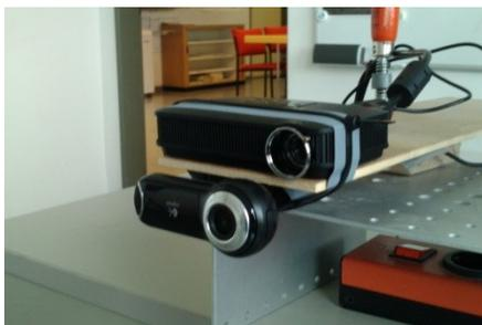
Figure 6: Test setup for virtual touch detection (mini LCD projector on top of a web cam).
