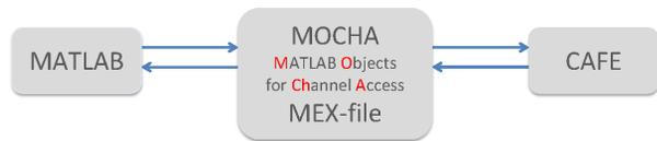
Figure 3: The MOCHA MEX-file provides the gateway from MATLAB to the CAFE library. Functions provided in the MEX-file are thus exposed to the MATLAB workspace.
