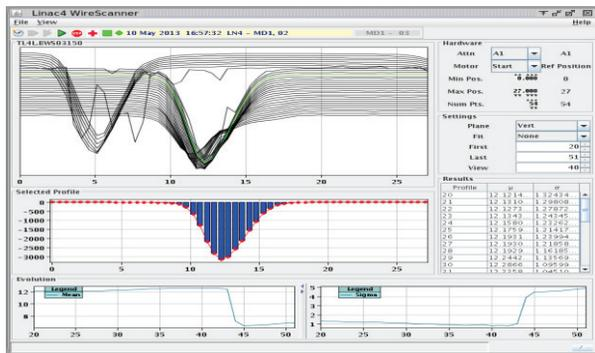
Figure 6: Profiles from the wire scanner while chopping which can be seen from the two distinct negative peaks in the distribution shown on the top.
