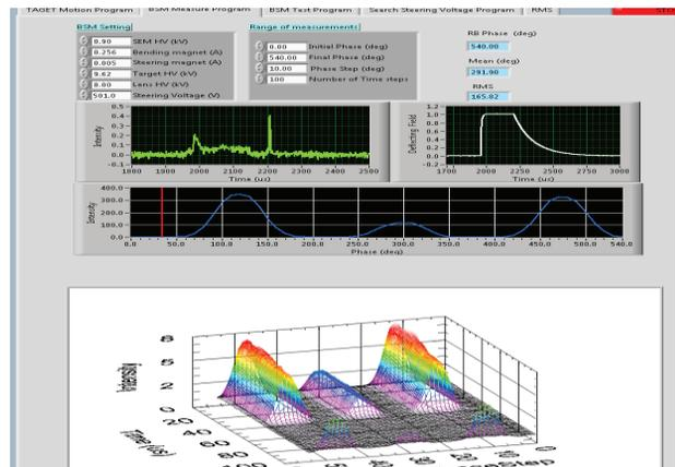
Figure 8: Bunch Shape Monitor LabView application. The lower plot shows the longitudinal beam distribution along the batch.
