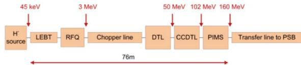
Figure 1: Overview of the Linac4 project from the H<sup>-</sup> source up the PSB injection transfer-line.
