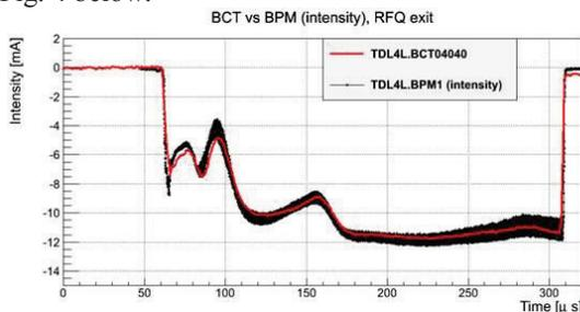
Figure 4: cross-calibrated intensity signal comparing signals from a BPM and a nearby BCT.
