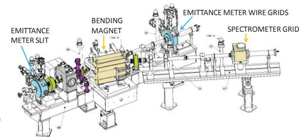
Figure 2: Schematic showing the measurement bench.
