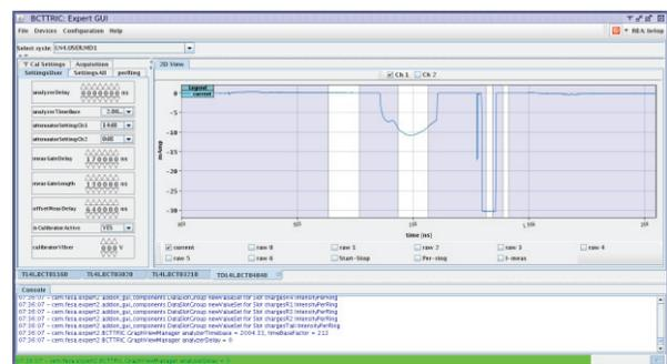
Figure 3: Java GUI allowing direct observation of beam intensity signals and the integration gates. The horizontal scale is in ns while the vertical scale is in mA.
