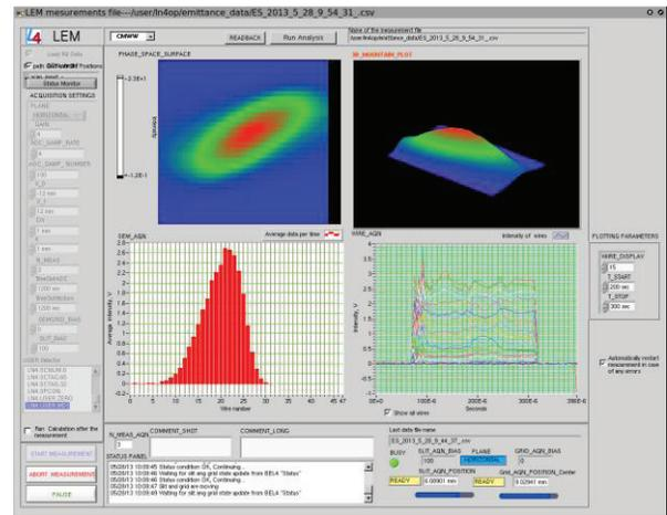
Figure 7: Transverse emittance-meter LabView application showing the emittance-meter results from 2D images to the projections.
