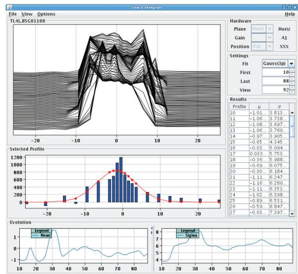
Figure 5: Transverse profiles measured with a Linac4 wire-grid. In the upper plot, the horizontal axis shows the position of the wires on the grid and the vertical axis shows the relative amplitude of the different acquired channels (some show hardware issues as can be seen more clearly in the middle plot).
