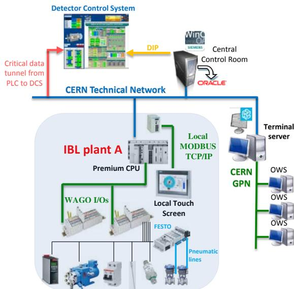
Figure 2: CO<sub>2</sub> cooling control system architecture.
