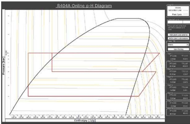
Figure 5: Real-time p-H diagram for R404a.
