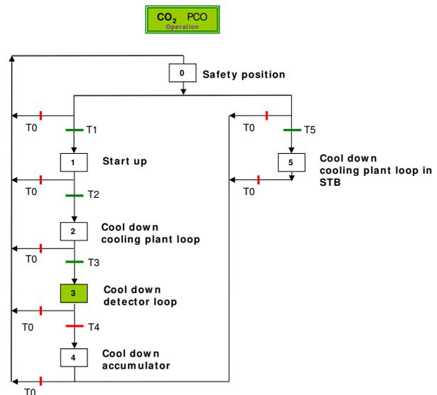
Figure 3: CO<sub>2</sub> cooling control system sequencer.
