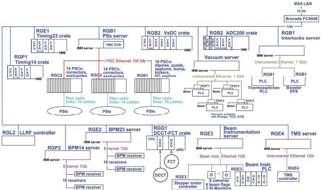
Figure 1: Block diagram of the equipment of the booster control system.
