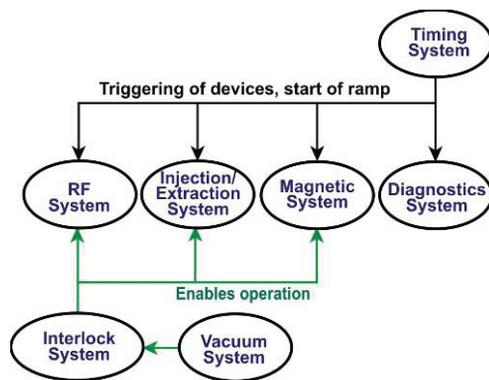
Figure 2: The booster control system interface diagram.
