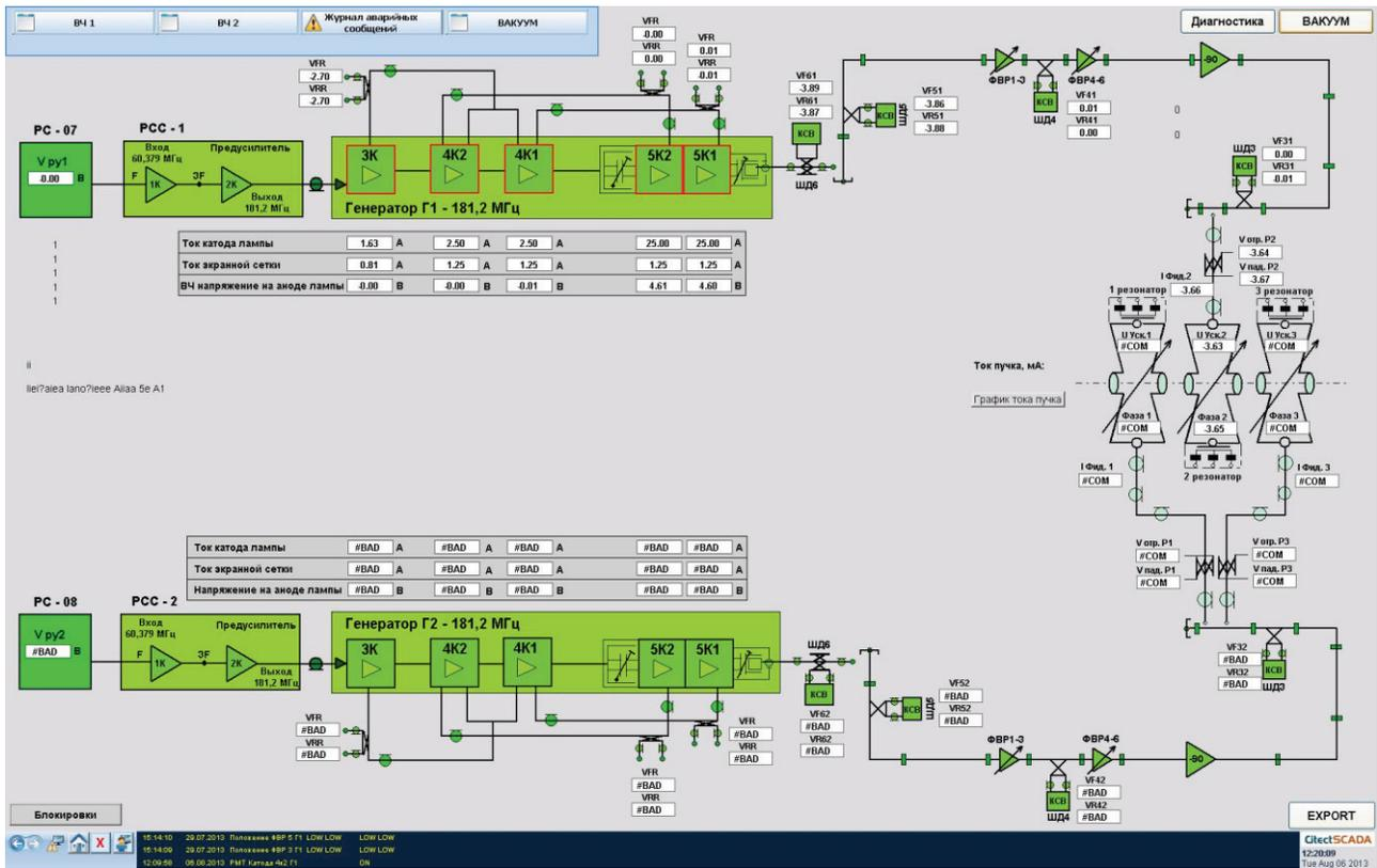
Figure 3: The video frame of functional diagram of RF-system of the main ring KRSRS.
