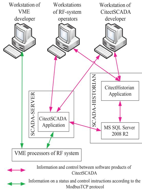
Figure 2: Functional structure of RF-generators CS.
