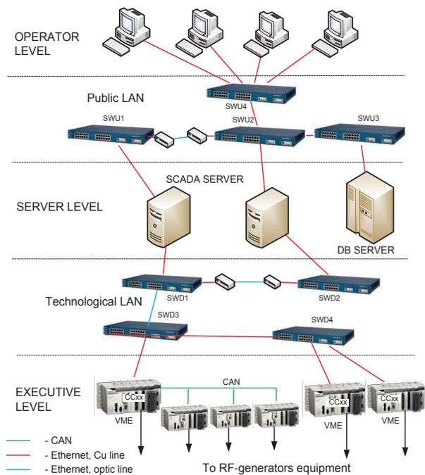
Figure 1: Structure of RF-generators CS.
