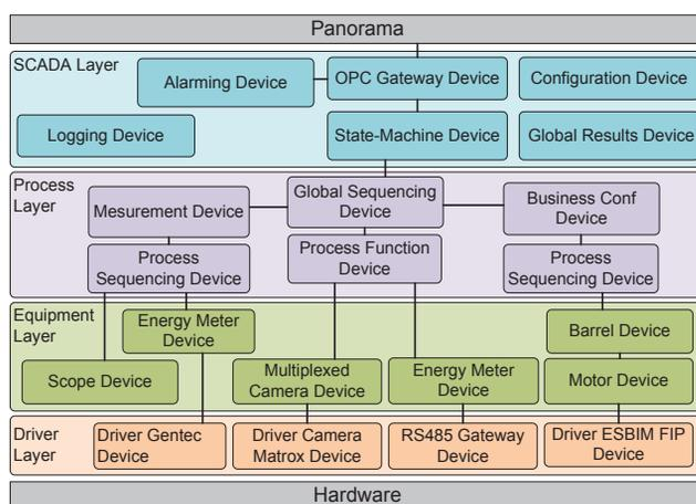
Figure 5: Four layer flexible architecture.
