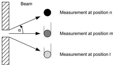
Figure 8: Measuring a beam profile for a single slit position.
