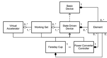
Figure 3: Class diagram of resources adapters for devices, Working Sets and Virtual Accelerators.
