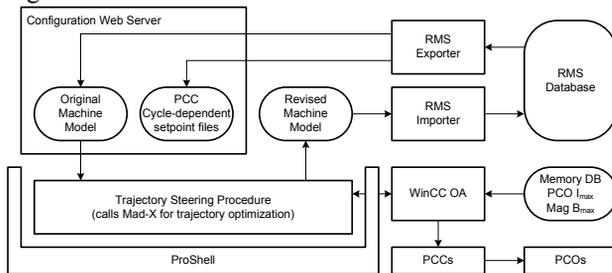
Figure 12: Basic data flow for trajectory steering.
