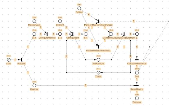
Figure 9: Petri net implemented by the phase space distribution measurement procedure.
