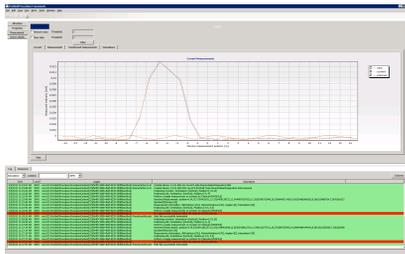
Figure 5: Single beam intensity measurement performed by a wire scanner.
