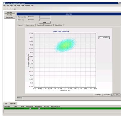
Figure 6: Combined phase space distribution measurement plotted over slit gap and wire position.
