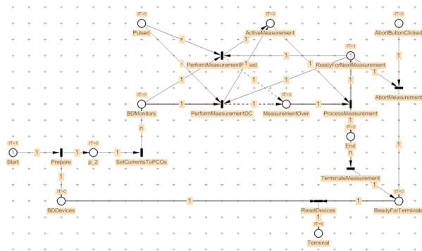
Figure 11: Petri net implemented by the trajectory steering procedure.
