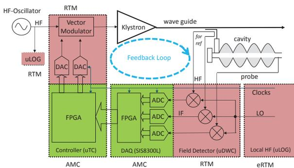
Figure 3: Typical accelerator control system layout based on MTCA.4 components
