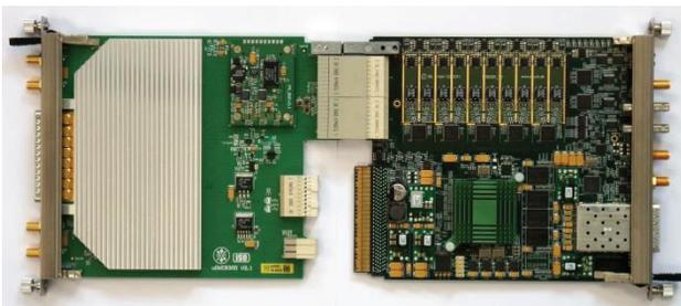
Figure 1: Pair of MTCA boards connected via Zone 3.
