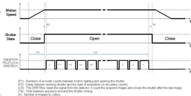
Figure 9: Timing of the most use triggering mode.
