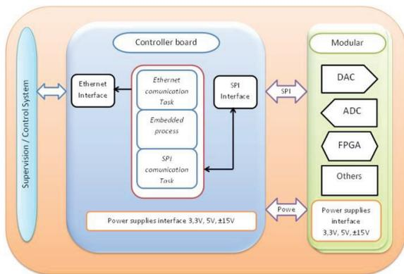
Figure 5: SPI Boards architecture.
