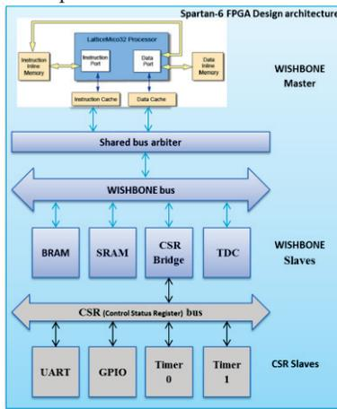
Figure 2: Demonstration design architecture.
