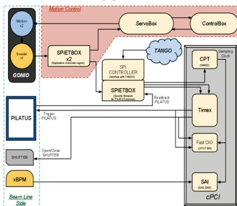
Figure 8: Architecture for PX1 acquisition with Pilatus.
