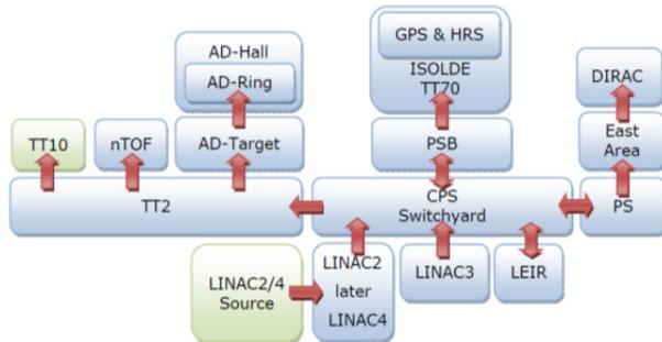
Figure 2: PS complex accelerator zones and beam paths.
