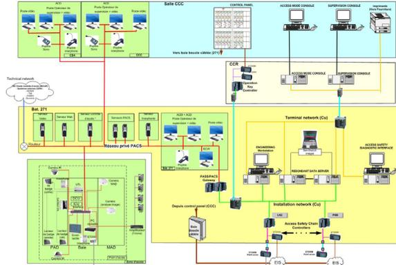
Figure 7: PACS and PASS integrated architecture.
