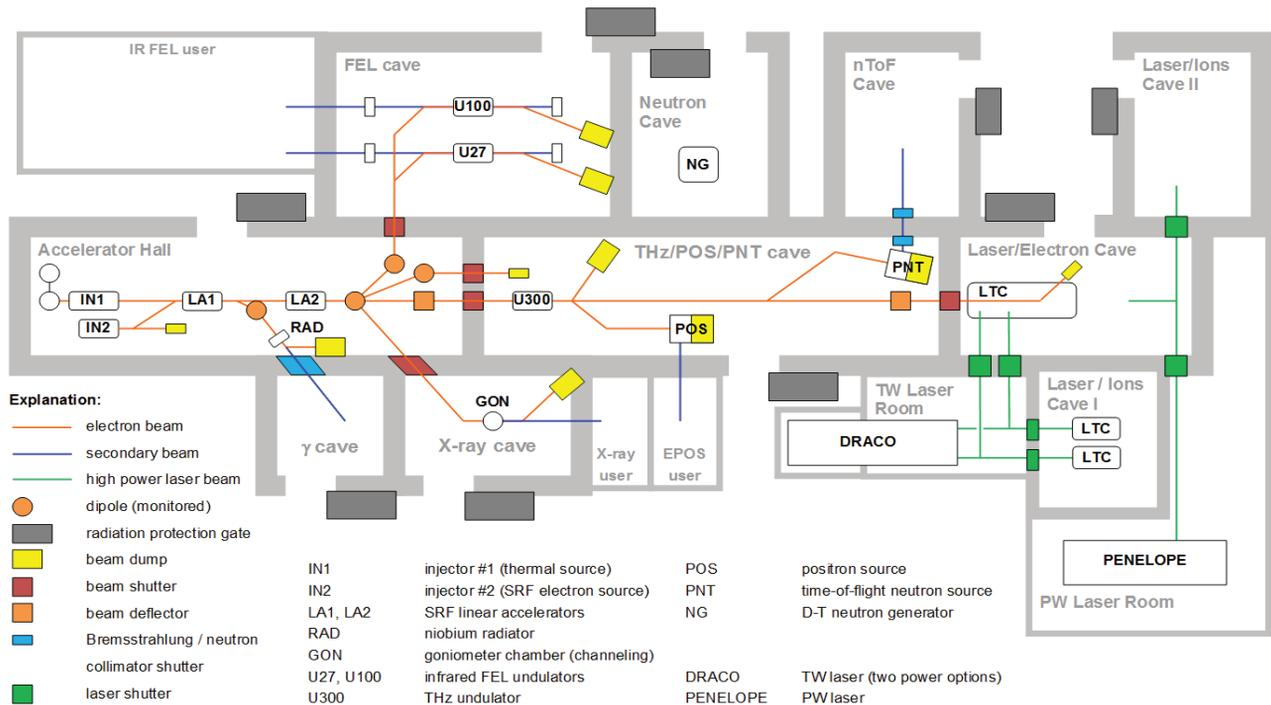
Figure 1: Overview of the ELBE Center for High Power Radiation Sources.
