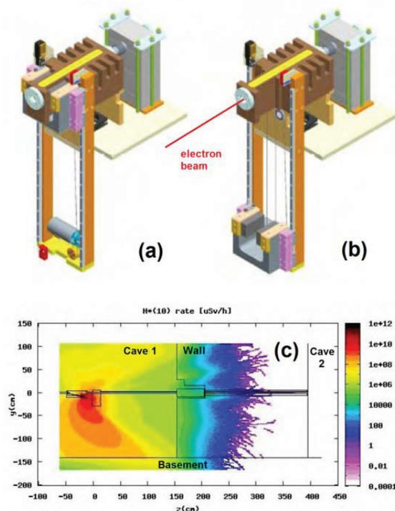
Figure 2: beam deflector for straight forward beam lines: (a) IN position (b) OUT position (c) radiation distribution from maximum beam power to be dumped.
