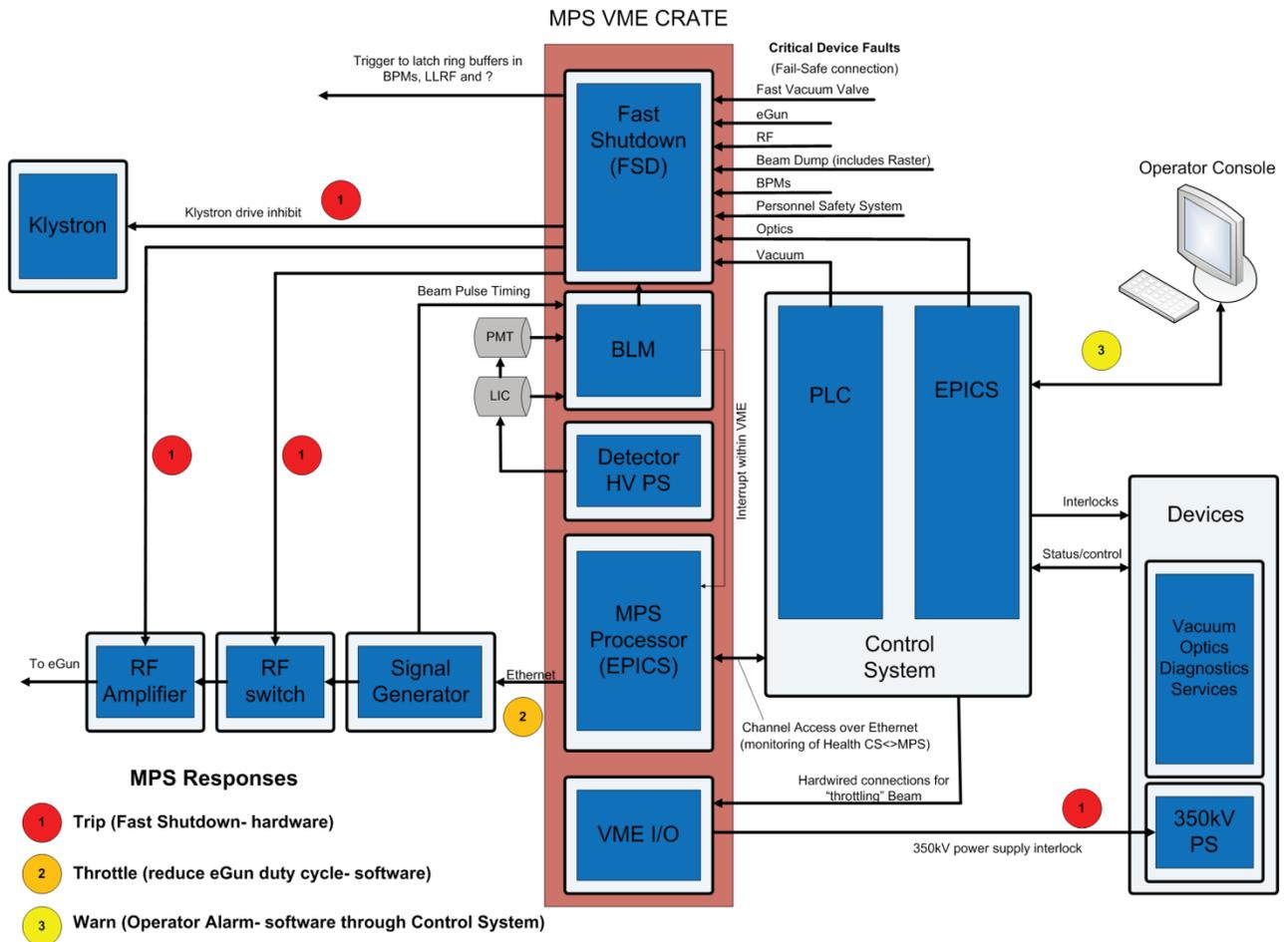
Figure 1: MPS Block Diagram.
