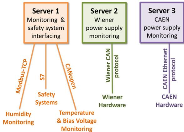
Figure 1: A diagram of the new CMS ECAL DCS architecture with the software running on three servers.
