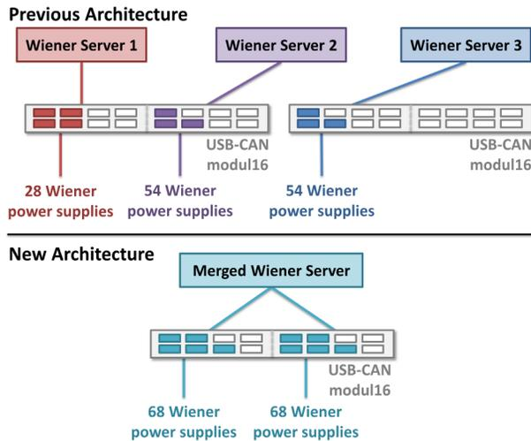
Figure 3: The interfacing of Wiener devices via USB and CAN in the old and new ECAL DCS architectures. Unused CAN ports are marked in white with grey outline.
