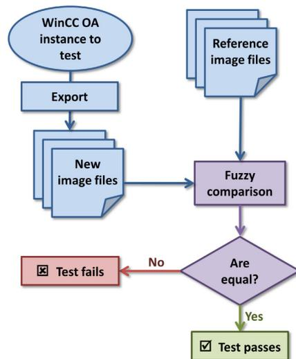
Figure 2: The procedure for validating a test instance of an ECAL DCS application against a valid reference.
