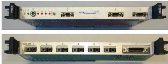
Figure 3: VICB8003 and transition module.
