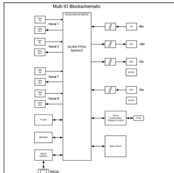
Figure 1: MULTI-IO block schematic.
