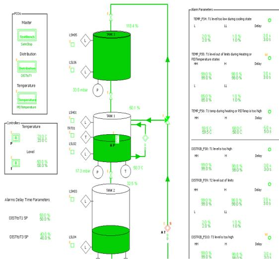
Figure 3: Water tanks process HMI.
