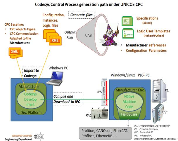
Figure 2: UNICOS-CPC CODESYS procedure.
