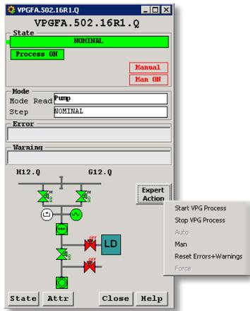
Figure 3: VPG6A Control Panel.
