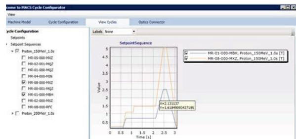
Figure 6: Settings generator showing waveforms for two magnets for one particular beam cycle.
