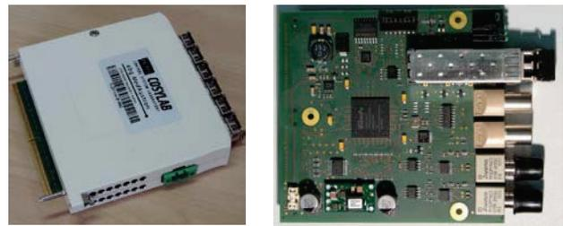
Figure 3: FlexRIO adapter (sender) and generic front-end device (FED) adapter board (receiver).
