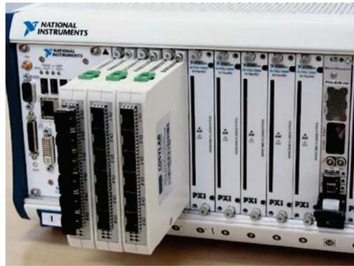
Figure 2: PXIe based frontend controller with FlexRIO cards, six port optical adapter and MRF event receiver cards.
