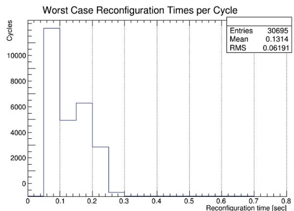
Figure 9: Observed worst case reconfiguration times of over 30 kCycles after code optimization.
