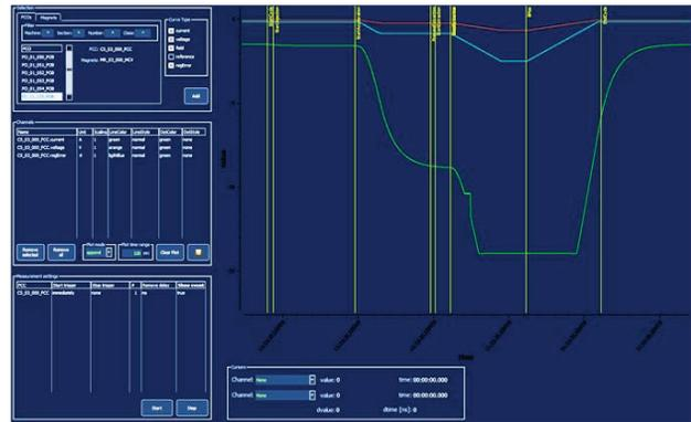
Figure 5: WinCC OA power converter control user interface panel with real-time display of timing events, generated waveform and regulation error.
