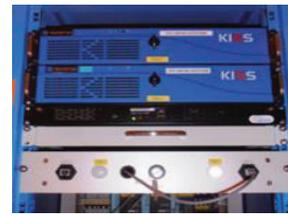
Figure 7: Redundant FESA (KISS) computers.
