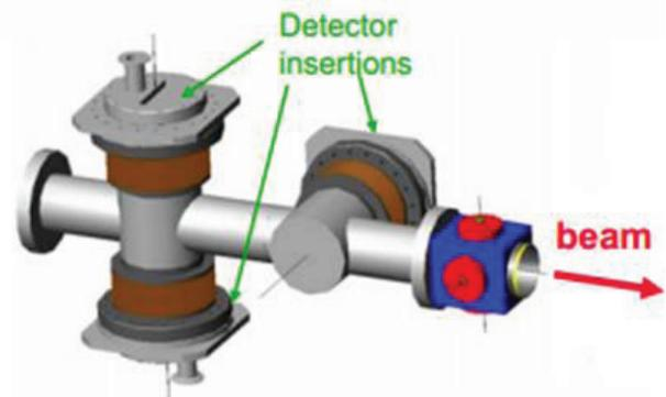
Figure 1: 2 Vertical and 1 Horizontal Roman Pot on the LHC beam pipe.
