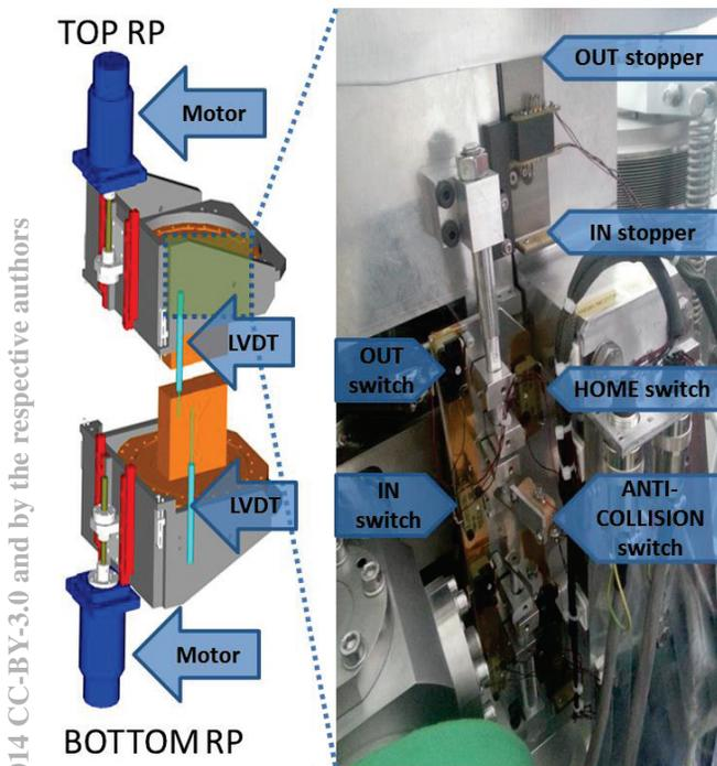
Figure 2: The Roman Pot Front End, sensors and actuators.
