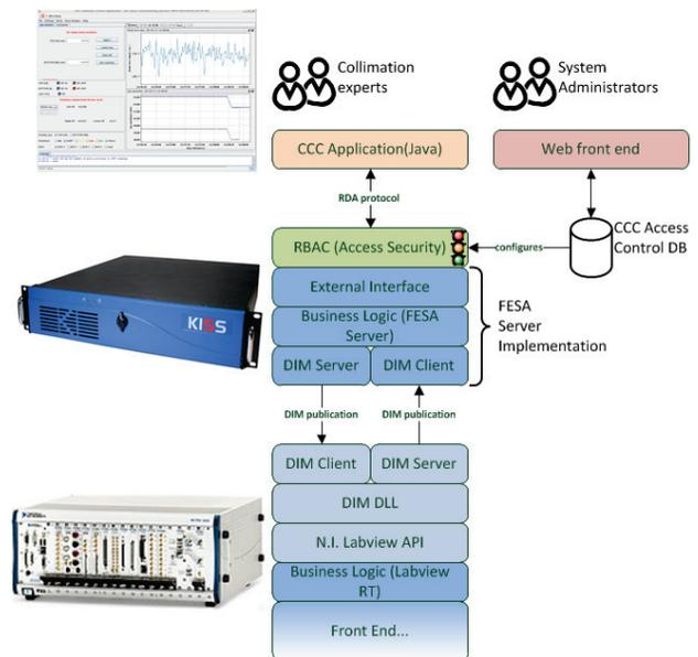
Figure 3: The control system back end and middleware.
